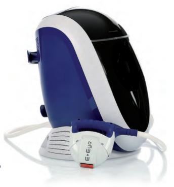
**E-EUQ** is a device that generates a new type of polychromatic pulsed light by producing perfectly calibrated and homogenously sequenced light pulses. The sculpted pulses are delivered under the shape of regulated train pulses. The energy, spectrum and time period are precisely set to stimulate the meibomian glands in order for them to return to their normal function.
